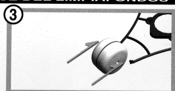
GB | Pull the skirt "B" down to the base of part "A" and clip it onto the groove.
