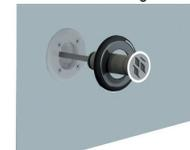
Insert the cable through the inlet and along the pipe.
